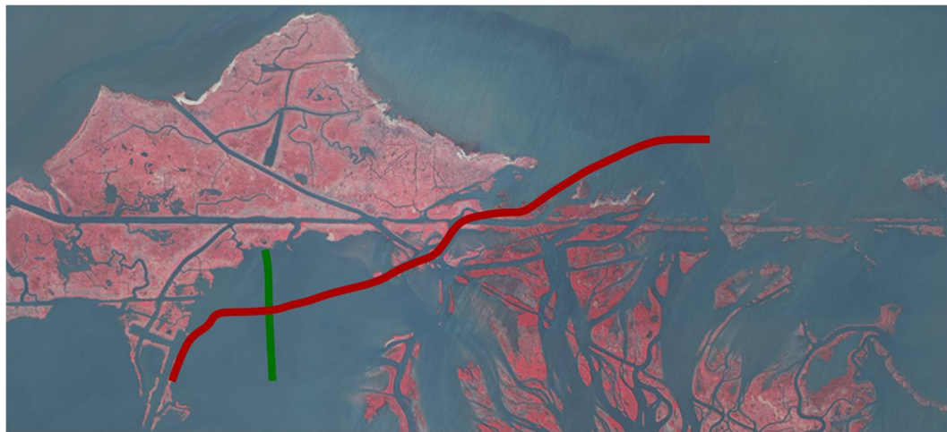
(b) .450s fault trace in red, and counter-regional fault trace, in green, layered over an orthophoto. Due to the shallow depth of the coherency data and the listric shape of the fault, the fault trace location better correlates to the location of the wetland.
