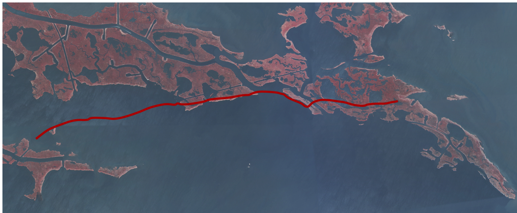
(b) .450s fault trace in red, layered over an orthophoto. Due to the shallow depth of the coherency data and the listic shape of the fault, the fault trace location better correlates to the edge of the wetland than the 1.0s trace.
