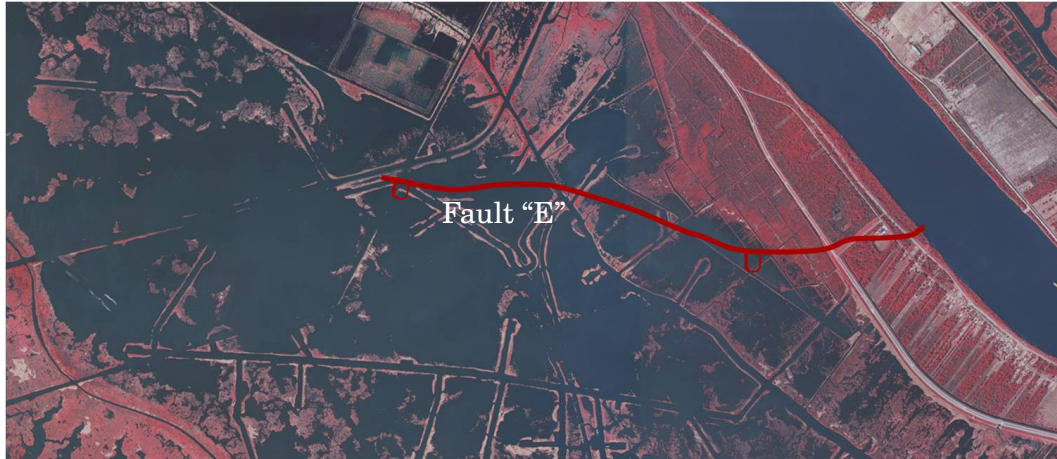
(a) 1.0s fault trace, in red, layered over an orthophoto. The location of the fault closely corresponds to the southerly extent of the marsh. Fault is suspected to continue to the West, however no seismic data was available to confirm this.
