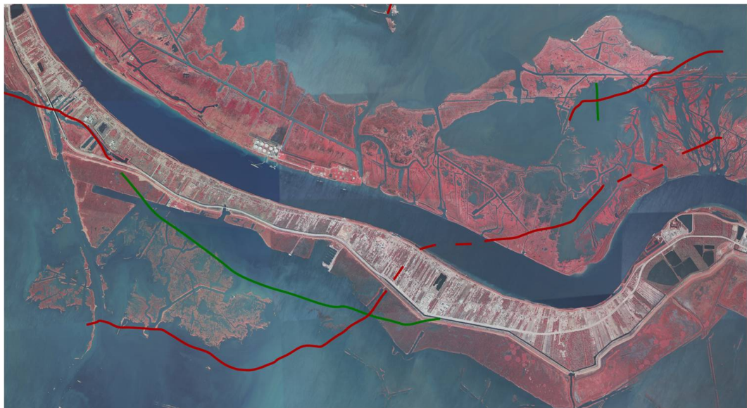
(b) .450s fault trace in red, and counter-regional fault trace, in green, layered over an orthophoto. Due to the shallow depth of the coherency data and the listic shape of the fault, the fault trace location better correlates to the locations of the wetlands and to the plan form of the Mississippi River.
