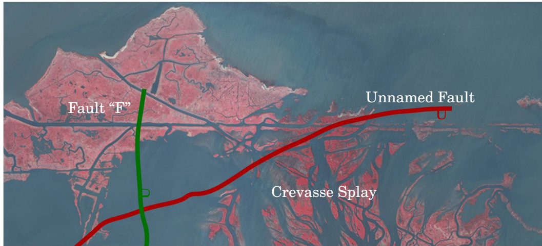
(a) 1.0s regional fault trace, in red, and counter-regional fault trace, in green, layered over an orthophoto. The locations of the faults roughly correspond to the location of the wetlands. Note crevasse splays filling space created by the hanging wall subsidence.
